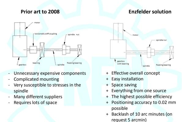
The company Enzfelder solves the problem with a hollow shaft, in combination with a special clamping system. This makes it possible to connect the motor directly to the gearbox and so there is no play between the motor and gearbox.
