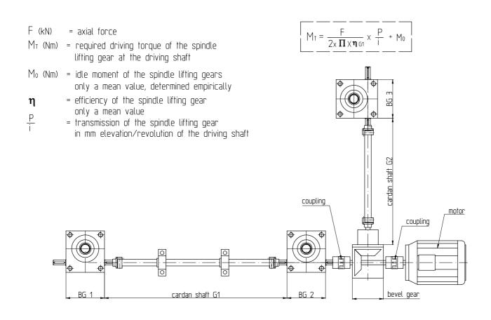
$$M_{\text{driving motor}} = M_{\text{T BG1 X}} \frac{1}{\eta_{\text{G1}}} + M_{\text{T BG2}} + M_{\text{T BG3}} \times \frac{1}{\eta_{\text{G2}}} \times \frac{1}{\eta_{\text{K}}}$$
