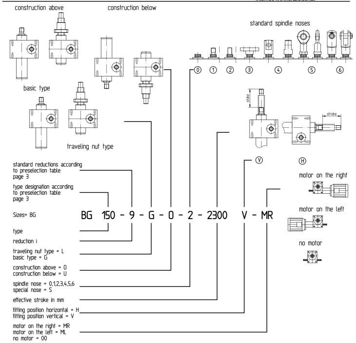
Above example for ordering: Sizes type 150, reduction 9:1, basic type construction up, spindle nose 2, stroke 2300mm, mounted vertical, with motor mounted on the right.
