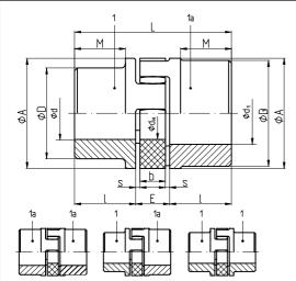
Finish-borings are made according, to the ISO system of tolerances H7. Feather key grooves are made according to DIN 6885/1. The max. angle shift is  $1^{\circ}30$ , the twisting angle  $3.2^{\circ}$  at M1 nom. The operable temperature range lies between  $-40^{\circ}\mathrm{C}$  and  $+100^{\circ}\mathrm{C}$
